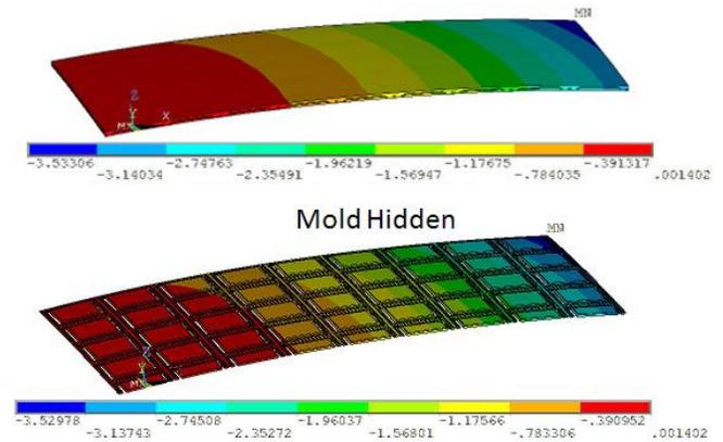
Figure 9. Strip panel warpage result in “frowning” mode after PMC (post mold cure).
