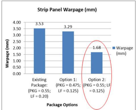
Figure 10. Strip panel warpage results comparison for the different options.
