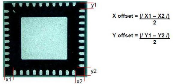
Figure 5. Illustration of how package offset is calculated.
