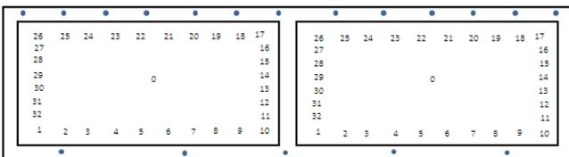
Figure 8. Warpage measurement points.
