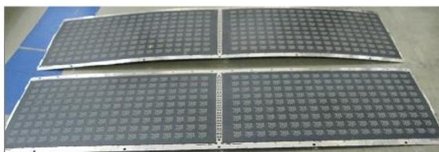
Figure 2. Ultra-thin QFN package molded array strip with “frowning” warpage at live bug position.
