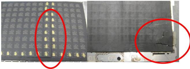
Figure 3. Molded strip showing package crack.
