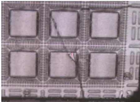
Figure 4. Strip with micro-crack.
