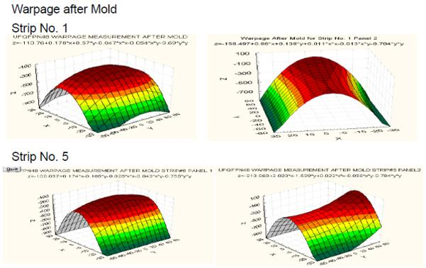
Figure 11. Strip panel warpage after mold.
