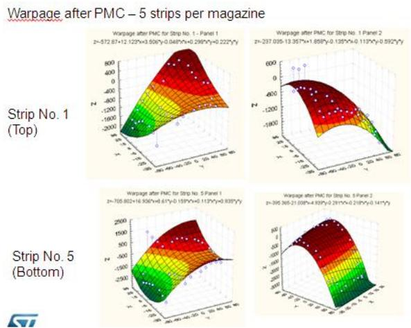
Figure 12. Strip panel warpage after PMC.
