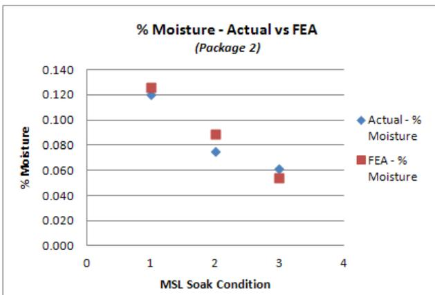
Figure 13. Package 2 - % Moisture (w/ EMC 2 & Glue)
