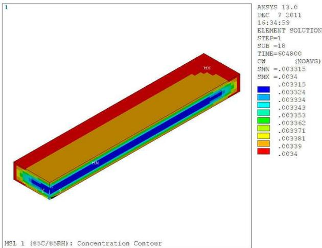
Figure 9. Moisture Concentration Distribution of the Bulk Molding Compound
