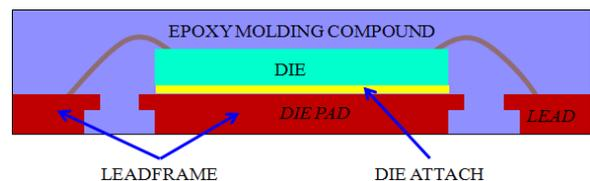
Figure 1. Schematic of the QFN Package
