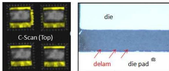
Figure 5. SCAT Photo and Cross Section of Package 1 (representative photo after MSL 1, 2 and 3)
