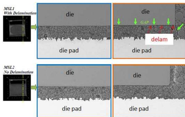
Figure 6. SCAT and Cross Section of Package 2
