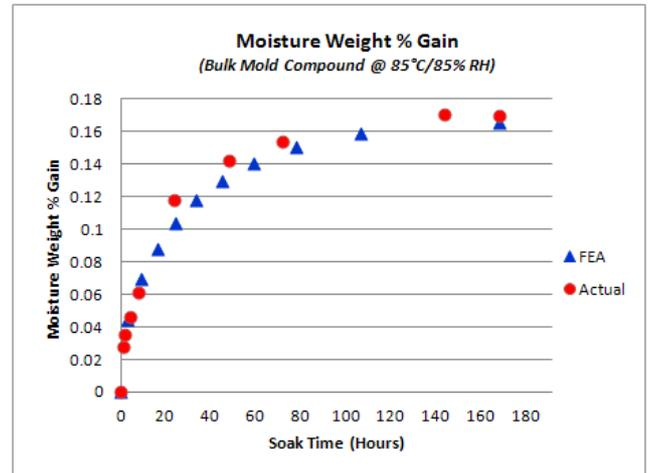
Figure 7. Moisture Weight Percent Gain of the Bulk Molding Compound (FEA vs Experiment)
