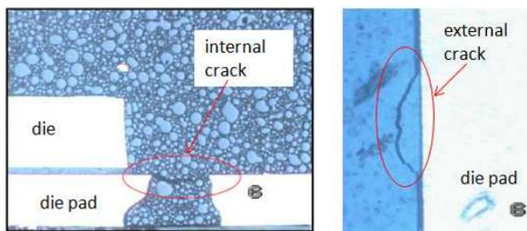
Figure 4. Cross Section of Package 1 revealing crack after MSL1
