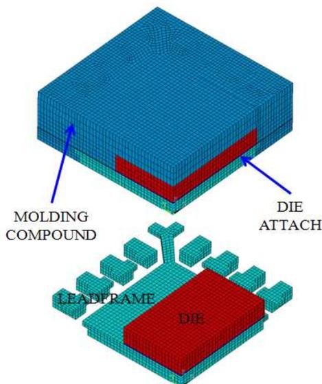
Figure 3. FEA Quarter Model of the QFN Package
