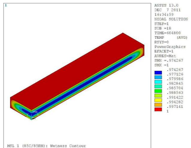
Figure 8. Moisture Wetness Distribution of the Bulk Molding Compound
