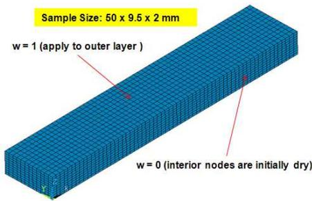
Figure 2. FEA Quarter Model of Mold Compound Sample
