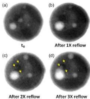
Figure 3. Growth of multiple voids after successive reflows<sup>2</sup>
