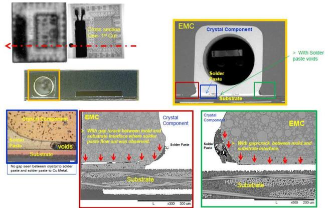
Figure 9. Cross-section results of the larger pad design (1<sup>st</sup> version with lead-free solder 1).
