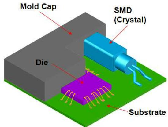
Figure 1. Schematic of a SiP with a large SMD.
