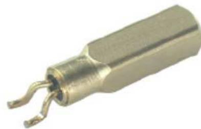
Figure 2. SMD Crystal with formed leads.
