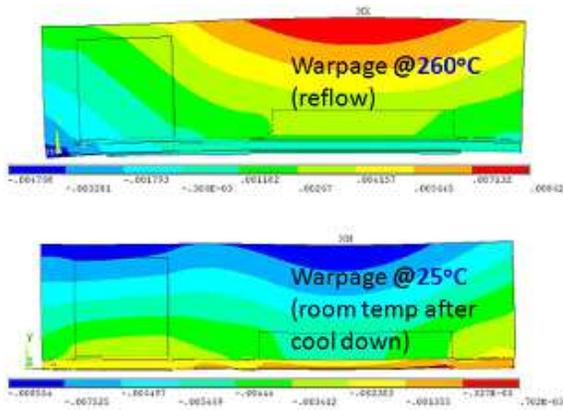
Figure 7. Package warpage at MSL reflow and room temperature.
