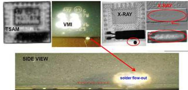
Figure 8. SCAT/visual inspection results of the larger pad design (1<sup>st</sup> version with lead-free solder 1).
