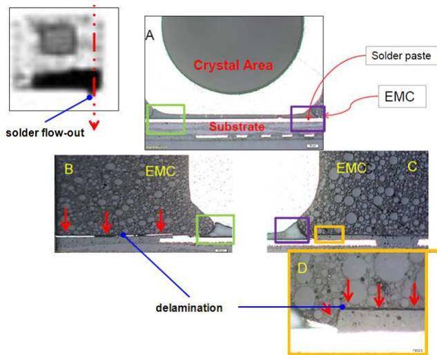
Figure 11. Results of the larger pad design (1<sup>st</sup> version with lead-free solder 2 – Evaluation Leg #2).
