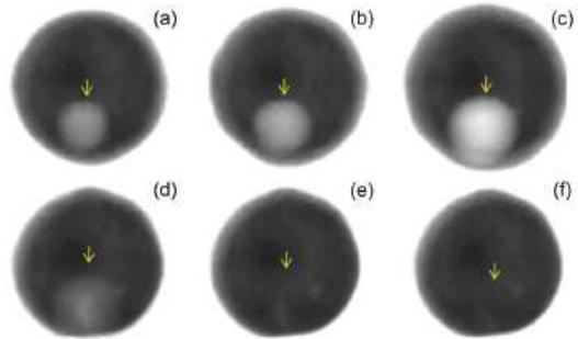
Figure 4. Popping of a solder void <sup>2</sup>.
