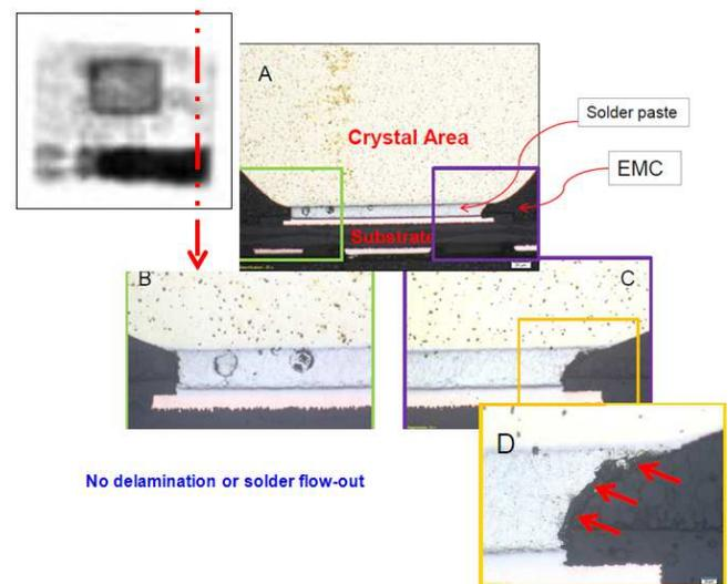
Figure 13. Results of the smallest pad design (final version with lead-free solder 2; Leg #6).
