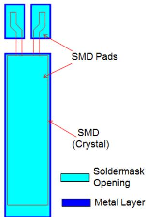
Figure 5. SiP Design (1<sup>st</sup> version with larger pad)
