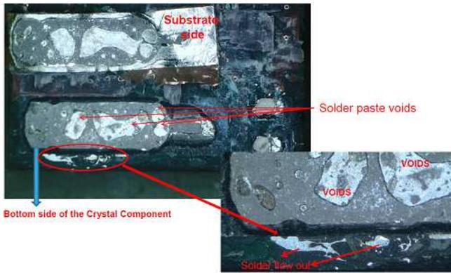
Figure 10. Mechanical decapsulation results (Evaluation Leg #1).
