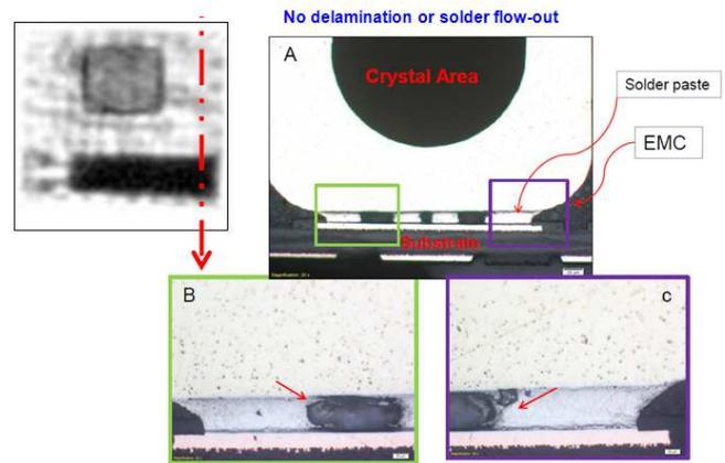
Figure 12. Results of the smallest pad design (final version with lead-free solder 1; Leg #5).
