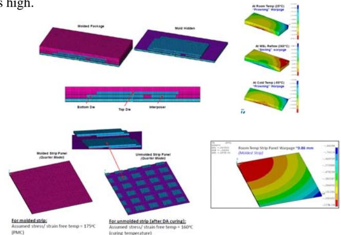
Figure9. UFLGA79 Thermo-mechanical simulations - package level and strip level.
