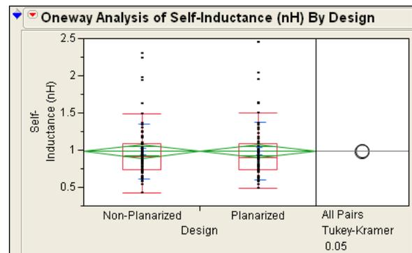
Figure14. No significant difference in self-inductances of all nets (signal traces + bondwires) between the two designs – Non-Planarized and Planarized.
