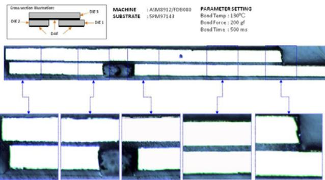
Figure11. Die attach stacked die using same rigid and thin DAF showed zero (0) voids for bottom dice at time (0).
