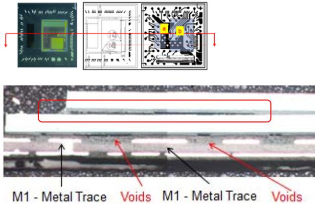
Figure7. Correlated metal trace plane serves as fulcrum and induces void, thus top delamination encountered.
