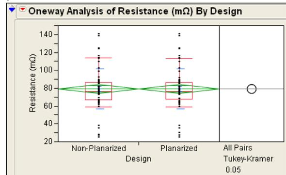
Figure13. No significant difference in resistances of all nets (signal traces + bondwires) between the two designs – Non-Planarized and Planarized.
