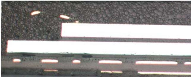
Figure10. Back-end assembly was performed using Softer and Thicker DAF for top die passed MSL3.
