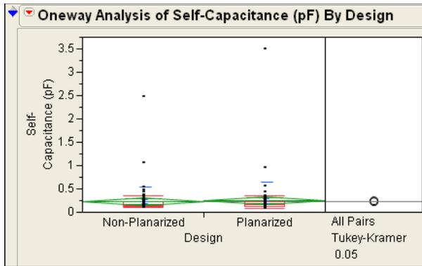
Figure15. No significant difference in self-capacitances of all nets (signal traces + bondwires) between the two designs – Non-Planarized and Planarized.
