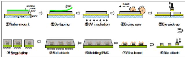
Figure3. General assembly flow with DDAF
