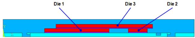
Figure 3. 2-D model of the QFN stacked die package (original design – baseline model).
