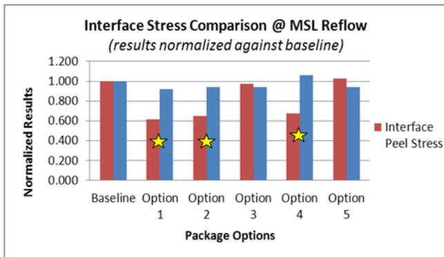
Figure 7. Interface stress results for the different package configurations.
