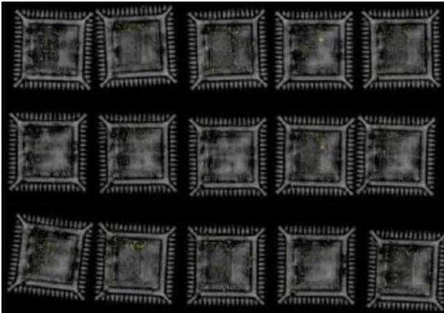
Figure 11. Scanning Acoustic Microscope (SAM) photo showing no delamination with roughened Ni.
