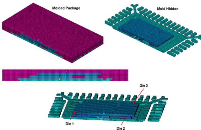
Figure 2. Finite element 3-D model of the QFN stacked die package.
