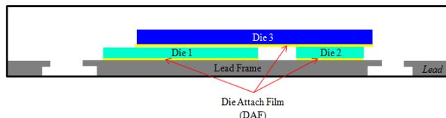
Figure 1. Schematic of the QFN stacked die package.
