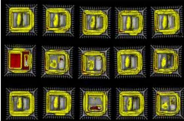
Figure 10. Scanning Acoustic Microscope (SAM) photo showing total delamination with PPF roughened by laser engraving.
