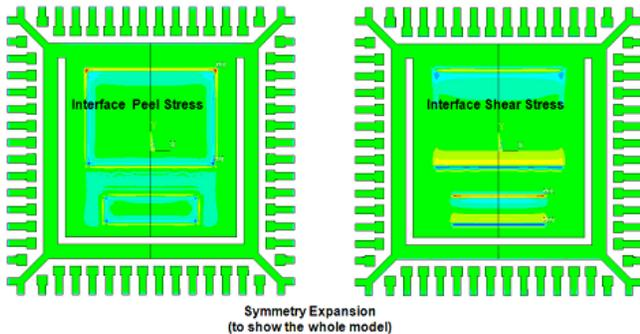
Figure 6. Lead frame interface (peel) stress result at MSL reflow showing high stress areas at the location of bottom die edges.
