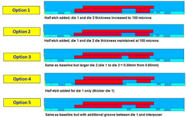
Figure 4. 2-D model of the different package configurations.
