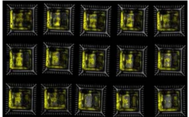
Figure 8. Scanning Acoustic Microscope (SAM) photo showing total delamination with the standard PPF.
