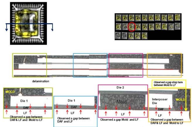
Figure 9. Cross-section photo confirming the delamination encountered.
