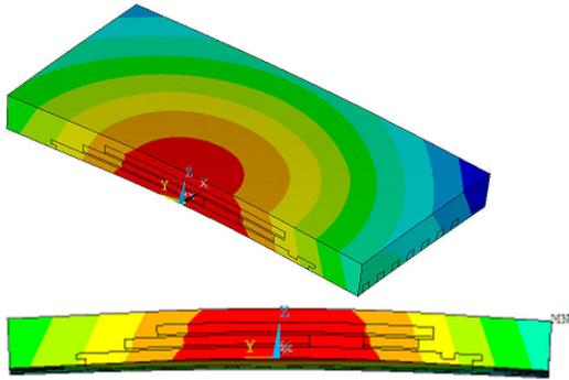
Figure 5. QFN stacked die package warpage result at room temperature (“frowning” mode).
