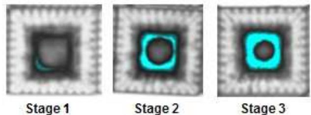
Figure 13. The development of delamination during thermal cycling.
