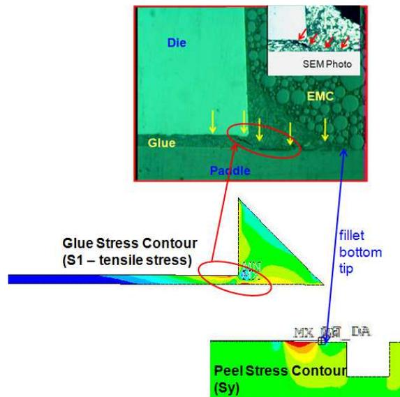
Figure 8. Actual delam/crack location vs stress results.
