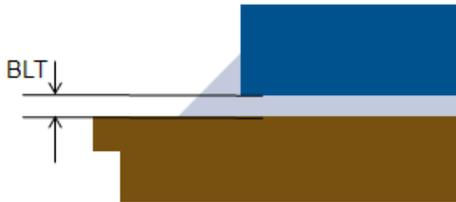
Figure 2. Bond line thickness (BLT) reference measurement.
