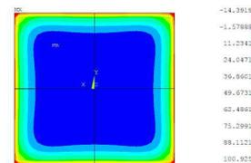
Figure 7. Glue stress contour plot of the 3-D model showing high stress areas at the edges.
