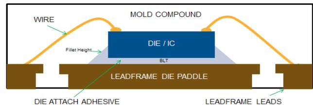
Figure 1. Cross-section drawing of a QFN package.
