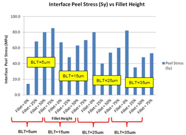
Figure 11. Interface peel stress simulation results.
