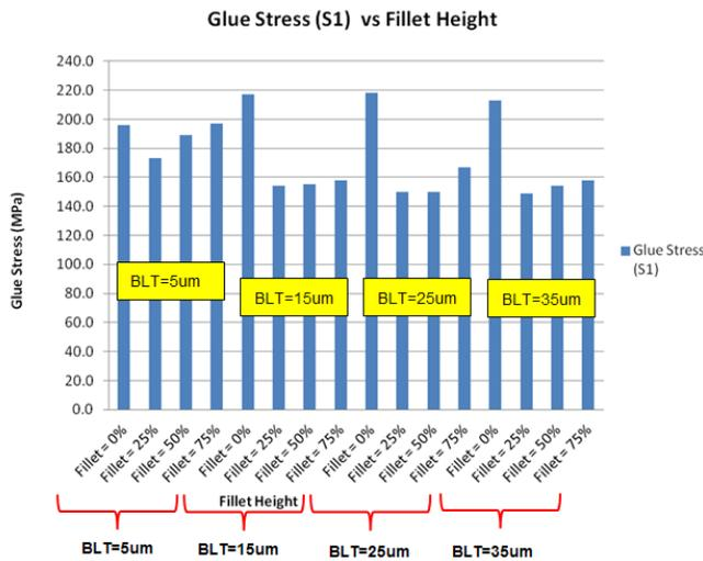
Figure 9. Glue tensile stress simulation results.
