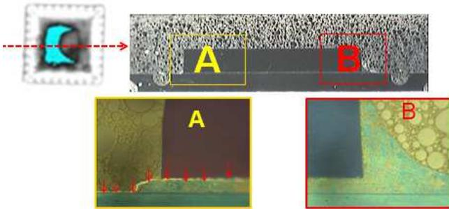
Figure 14. Cross-section and SEM photo of a sample unit with delamination.
