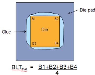
Figure 3. Measuring BLT during in-line assembly process.
