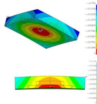
Figure 6. Warpage contour plot of the 3-D showing “frowning” warpage.
