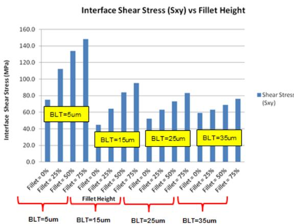
Figure 10. Interface shear stress simulation results.
