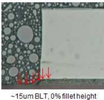
Figure 15. Cross section result of unit with ~15 $\mu\text{m}$  BLT and ~0% fillet height.
